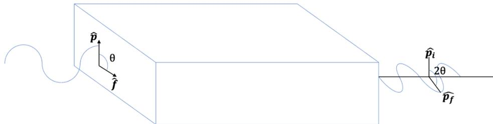
**Figure 1.** *Half waveplate diagram.* Vectors described below.
