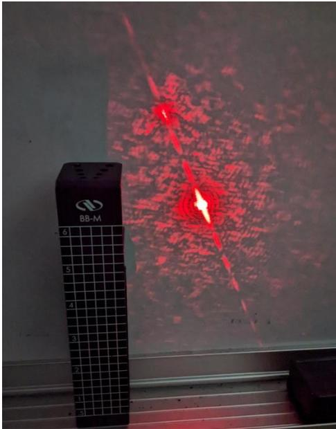
**Figure 12.** *Hair diffraction pattern.* The distance from peak to peak was measured, this, combined with the other factors allowed the calculation of my hair width.
